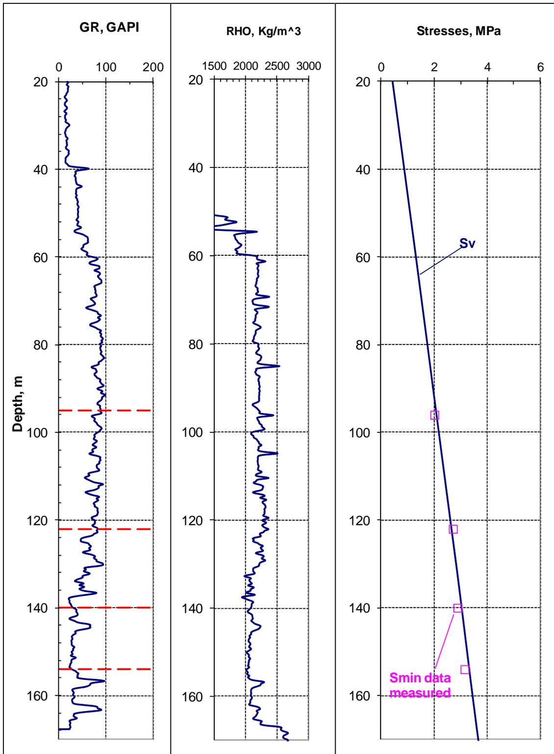
**Figure 1:** Summary of the in-situ minimum stresses measured from Well 07-25. Red dotted lines on the gamma log denote the mini-frac test intervals. “Sv” denotes the vertical overburden stress calculated from the density log. “Smin” in squares is the interpreted minimum stress from the mini-frac tests.
