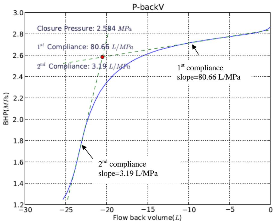
Figure 6: Fracture closure pressure interpreted from the compliance plot for Cycle #2 in the McMurray shale test at 122-122.5 m. The negative volume on the x-axis denotes the flow-back volume.
