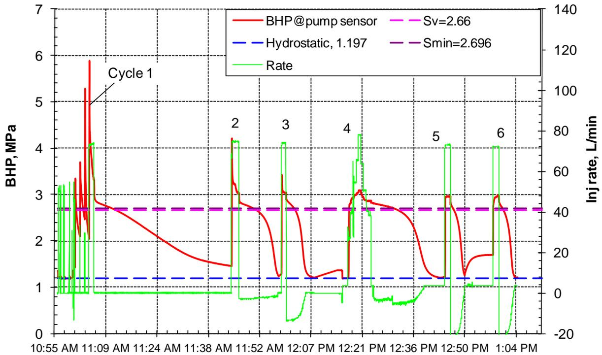
**Figure 3:** Pressure/rate history, McMurray Shale at 122-122.5 m TVD.
